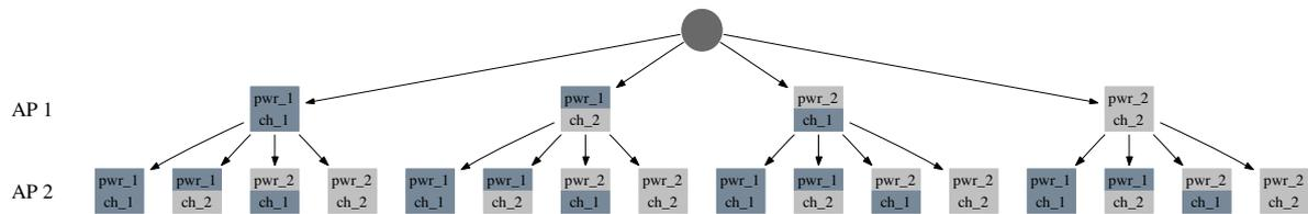
Figure 6.1: Branch-and-bound tree: joint channel and power optimization
