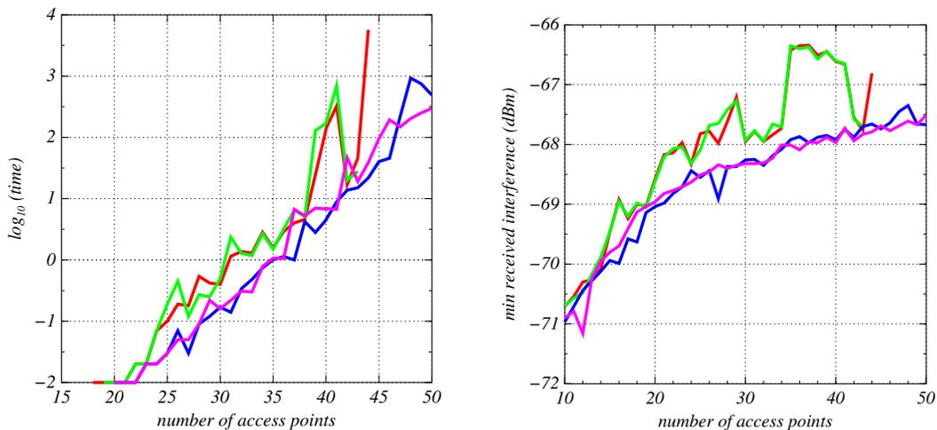
Figure A.2: The computational time and minimum received interference in a channel allocation problem for 4 different quasi-random algorithms: **Niederreiter**, **Sobol**, **Halton** and **reverse Halton**.
