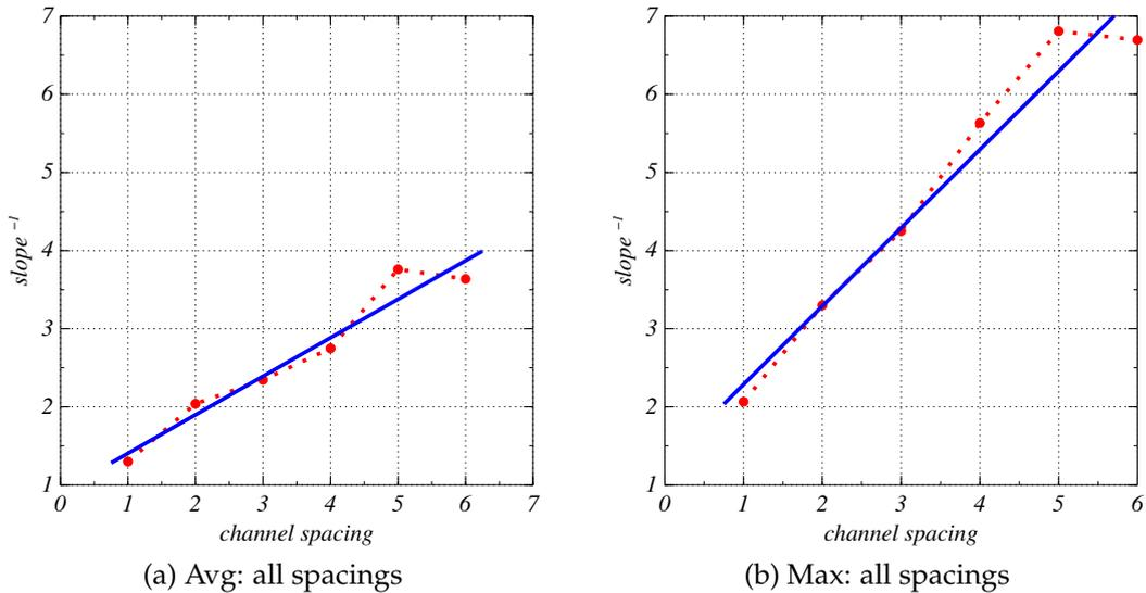
Figure 5.4: Relation between  $\text{slope}^{-1}$  and channel spacing, where  $\text{slope}$  is the slope of the computational time versus the number of access points on a logarithmic scale. See also Figure B.1 and B.3
