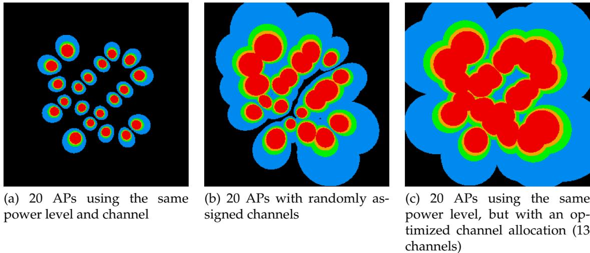
Figure 5.3: Comparison in throughput and coverage using a single channel, a random assignment or channel optimization with 13 channels, showing mode 1, mode 2, mode 3, mode 4 and no throughput. The modes are defined in Section 4.1.3
