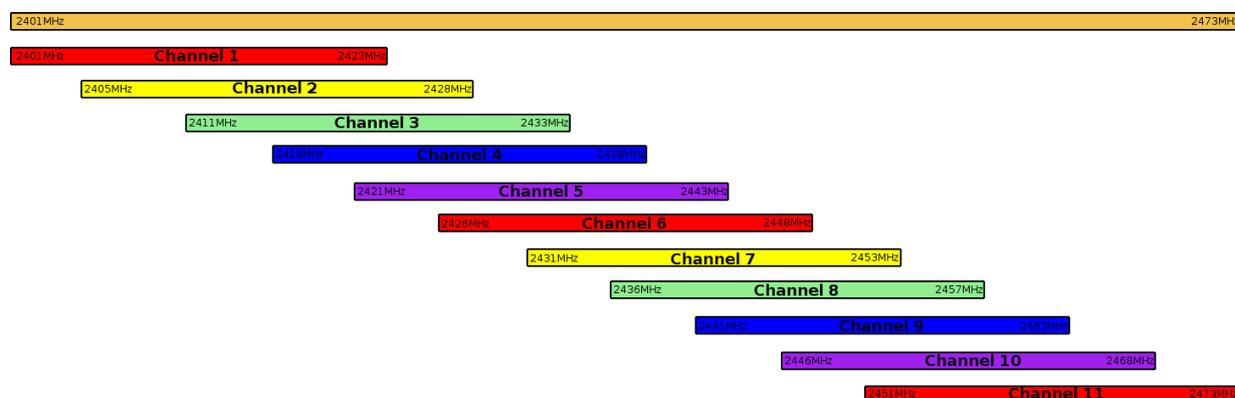
Figure 4.1: Spectral channel overlap in IEEE 802.11b (US channels)
