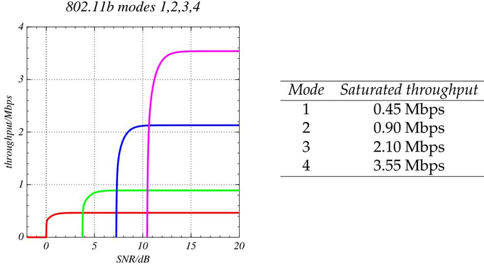
Figure 4.2: Throughput for 4 different modulation schemes in IEEE 802.11b [3]
