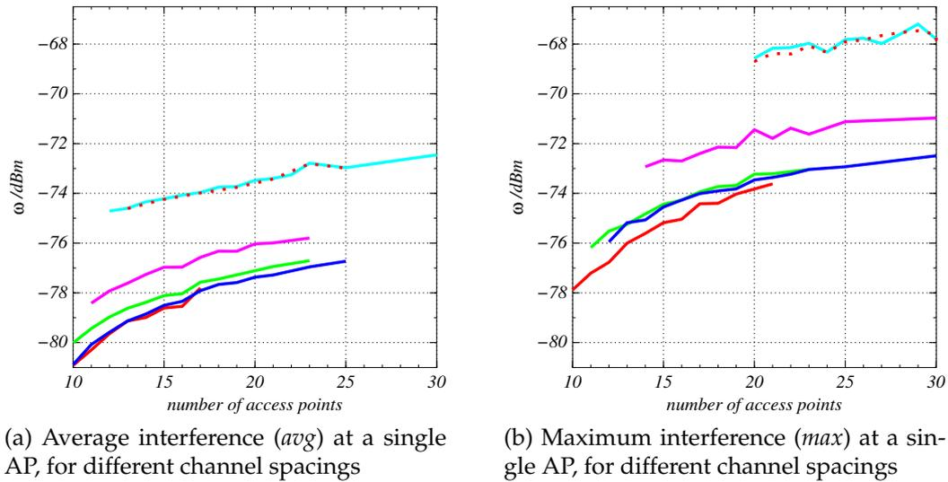
Figure 5.5: Received interference at a single AP, when optimizing the *sum* or *max* objective, for channel **spacing 1**, **spacing 2**, **spacing 3**, **spacing 4**, **spacing 5** and **spacing 6** (dotted)
