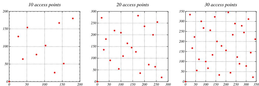
Figure A.1: Quasi-random generated access points locations, using the Niederreiter algorithm
