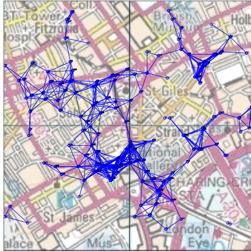
Figure 7.3: Soho interference graph that connect potential interfering access points
