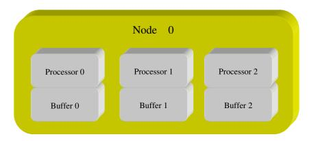
Figure 4.1: Node hardware architecture and naming method
