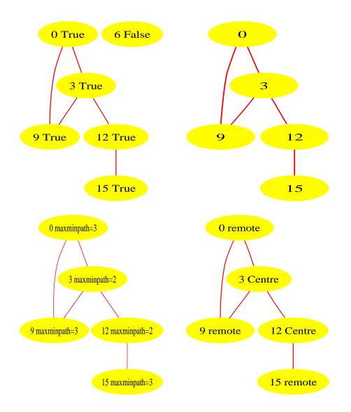
Figure 4.8: Process of the program: top left: Result of connectivity; top right: Return the connected partition; bottom left: Compute the eccentricity; bottom right: Compute the center
