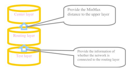
Figure 4.5: Message passing between layers inside the node
